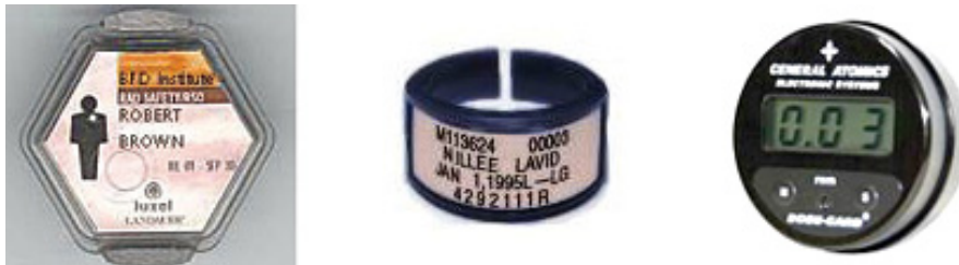
Dosimeters: film badge (left), ring badge (center), and real-time (right). (Sources: OSHA and U.S. DHS.)
